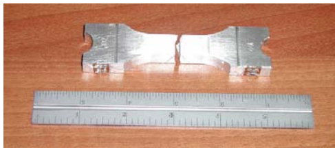
Corner Crack Tension, CC(T)
