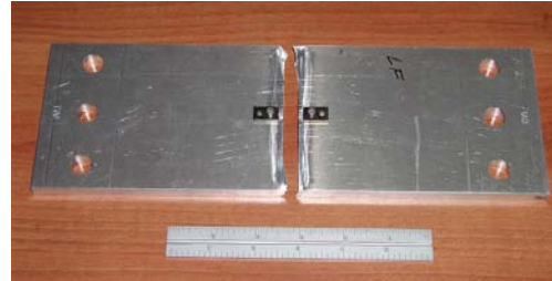
Middle Crack Tension, M(T)
